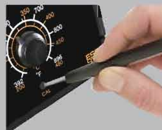
The fine-tuning temperature of soldering station is controlled by tools.
